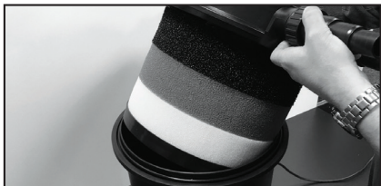
Step 5 - Lift the lid and connected sponges out of the filter body and turn upside down
