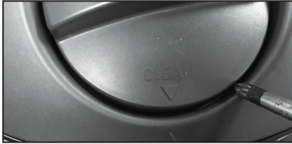
Step 1 - Prize off the valve with a screwdriver. ENSURE POWER IS SWITCHED OFF.
