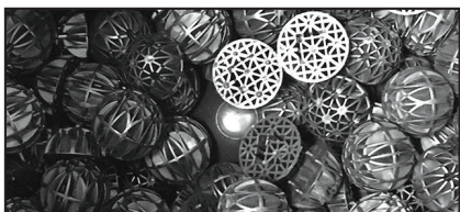
Step 9 - To clean black Bio Balls in the base of the filter, remove by hand and wash in old pond water, then replace.
