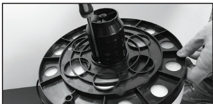
Step 7 - Using a screwdriver (not supplied) undo the screws in the bottom support plate.
