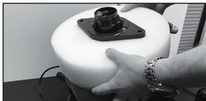
Step 8 - Sponges can then be lifted off and replaced.
